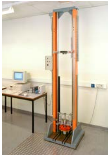
Home build impacter
