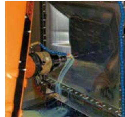
A finger like tool is run over a flat metal plate and creates a 3-dimensional shape by plastic deformation
