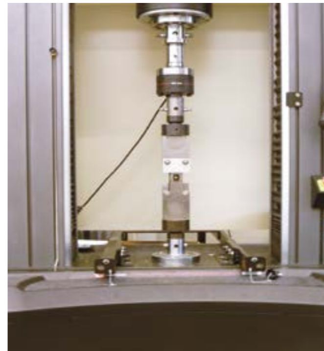
(below left) Open hole compression setup and (below right) Compression after impact
