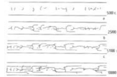
Damage history on the replicas taken after several fatigue cycles (PhD thesis of Martine Wevers)
