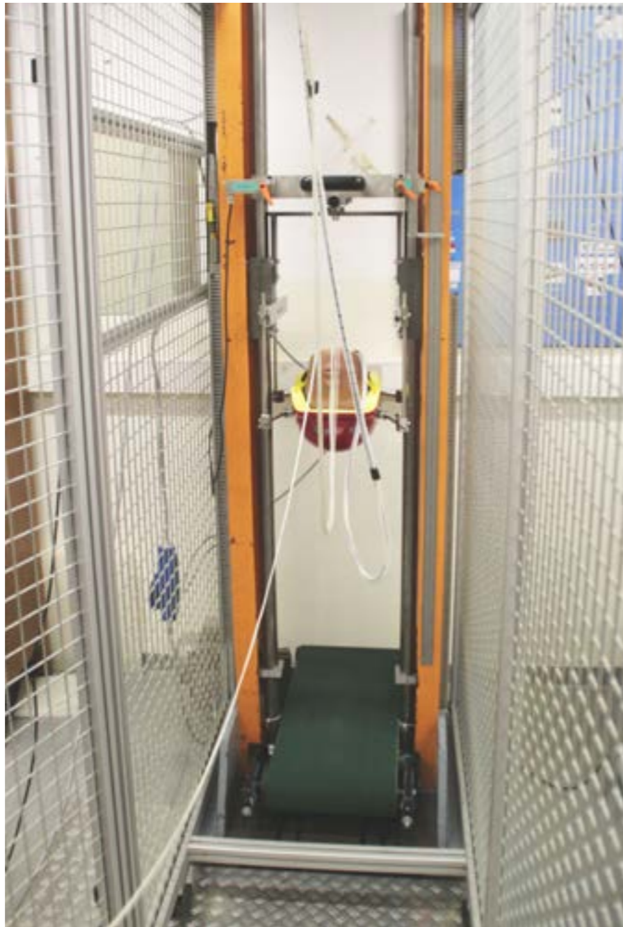
Home made helmet tester with dummy head and rotating belt as bottom plate to realistically mimick oblique impacts
