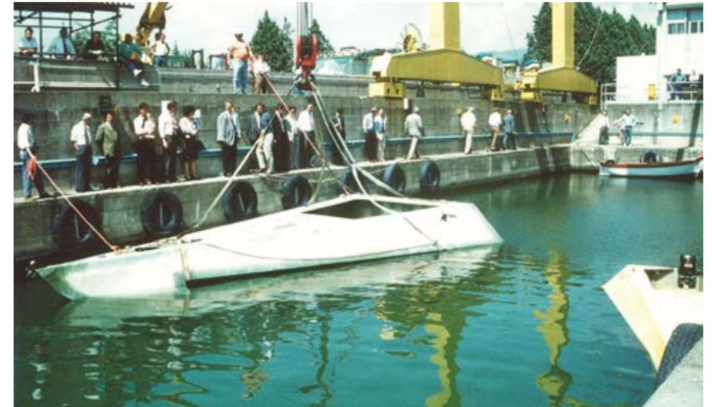
The AFICOSS-partners on the quay of Intermarine, admiring the experimental patrol boat for the Italian financial police, entirely made out of 3D-woven fabric composites
