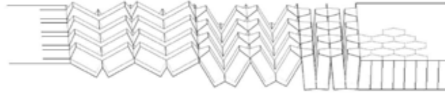
The production principle of the Thermhex thermoplastic honeycombs: vacuumforming half-hexagonal shapes, then longitudinal folding.
