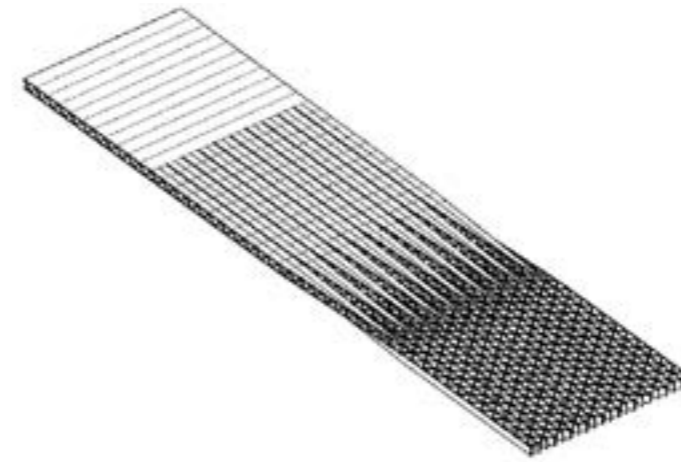
The production principle of the Torhex paper honeycombs: longitudinal slitting of a corrugated cardboard, then rotating over 90°
