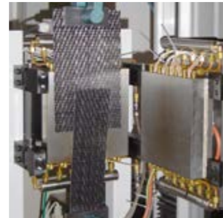
(above) Device for measuring interply friction at high temperature, a useful device for simulations of thermoplastic composites (right) Picture frame test setup for characterization of the draping behaviour
