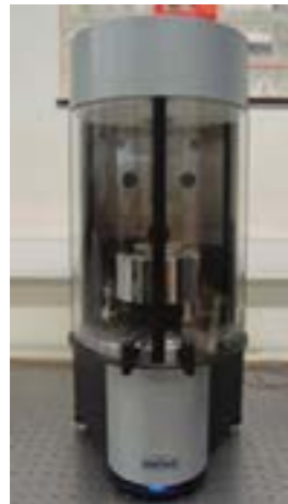
(below) Small tensile machine for single fibre testing and Tensiometer
