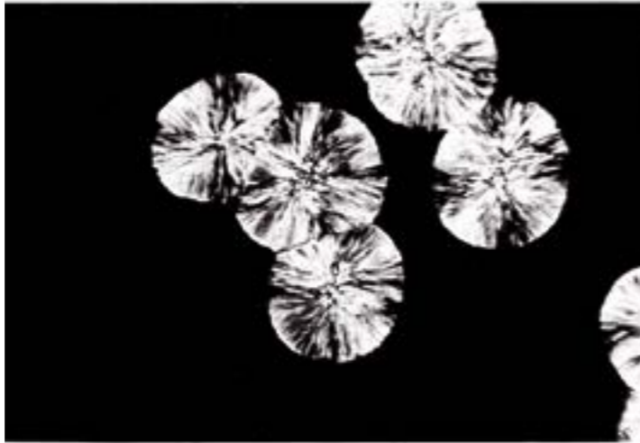
Spherulitic microstructure of PAA(poly-aryl-amide) (PhD thesis of Bernard Goffaux)
