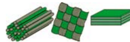
Three hybridization strategies for combining brittle and ductile fibres: intrayarn, intralayer and interlayer
