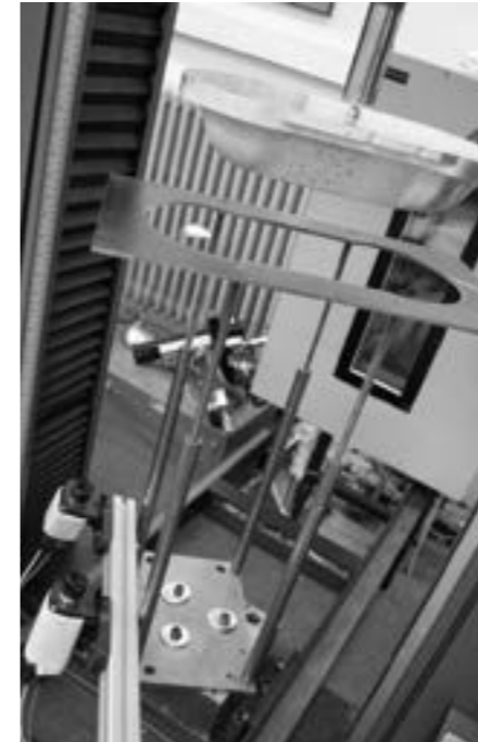
Test setup for studies of textile reinforcement draping with mould at the top and DIC-cameras at the bottom left
