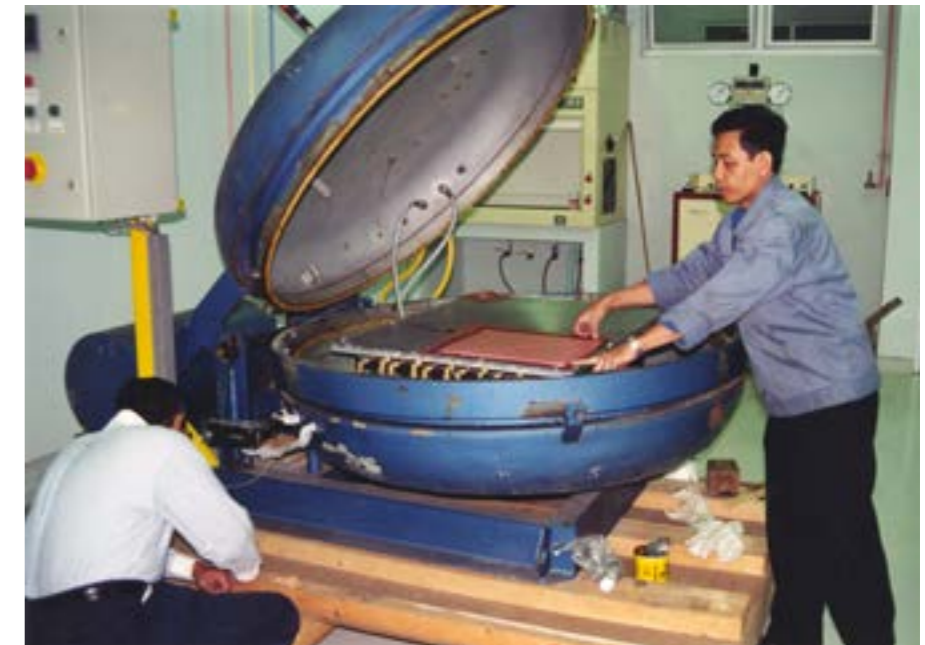
The heat exchanger of EBES converted into an autoclave (above) and Bandag autoclave installed in Indonesia (below)
